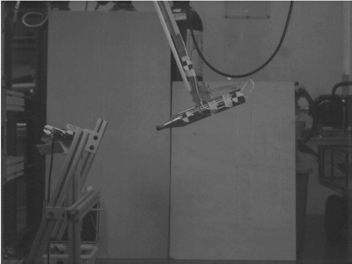
Figure 4.33: Pendulum impact frame setup image showing mass tip in freefall.
