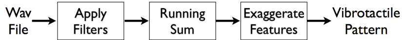
Figure 1. Block diagram showing the process of converting a wav file to a vibrotactile pattern
