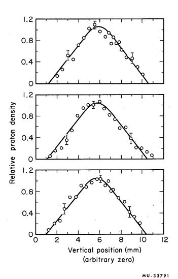
Fig. 17. Vertical scan of three different emulsions at random horizontal positions to determine the beam width. The lines are to guide the eye.
