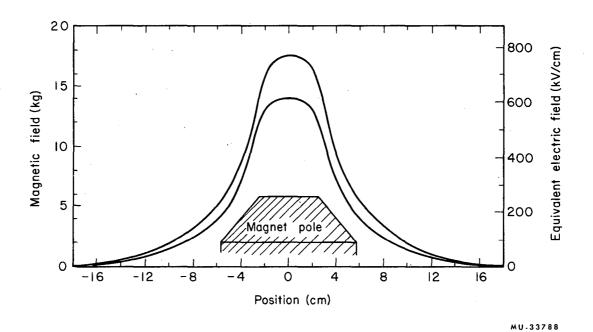
Fig. 12. Typical magnetic-field profiles, measured along the beam line, of magnet LM2 for two
