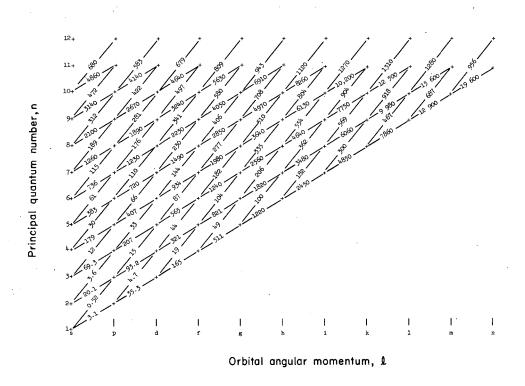
Fig. 4. Collisional excitation cross sections for 10-MeV hydrogen atoms incident on an electron target, based on the results of McCoyd and Milford.  $^{24}$  The numbers on the lines connecting the various states are the cross sections for the indicated  $n, \ell \rightarrow n+1, \ell+1$  or  $n, \ell \rightarrow n+2, \ell+1$  transition, in units of  $10^{-18}$  cm<sup>2</sup>. (Theoretical)
