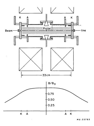
Fig. 8. Diagram of the PIG discharge-target chamber (drawn to scale). The dashed line indicates the shape of the right-angle probe used for longitudinal density measurements (Fig. 11); it was located at an azimuth of 45° to clear both the radial probe and the microwave horns. The curve below the diagram shows the shape of the magnetic field produced by the coils.
