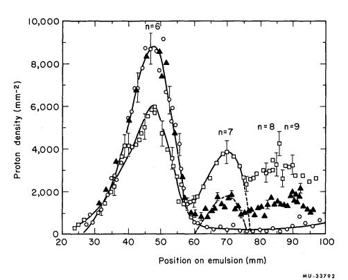
Fig. 18. Change in population of the levels n = 6 to 9 due to collisions with H<sub>2</sub>. All levels above n\* = 6 of the incident beam were depopulated by Lorentz ionization in LM1. Pressure in target: 0, 5×10-5 torr (evacuated target);
