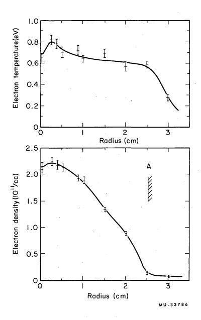
Fig. 10. Langmuir-probe measurements for the radial profiles of electron temperature and density in the PIG target. The error bars are based on reproducibility only (Hydrogen gas; pressure, 11×10<sup>-3</sup> torr; applied potential, 400 V; discharge current, 1.3A; magnetic field at center, B<sub>0</sub> = 260G).
