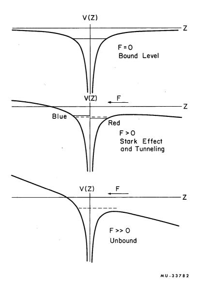
Fig. 1. Distortion of the electronic potential of a hydrogen atom caused by an electric field F.
