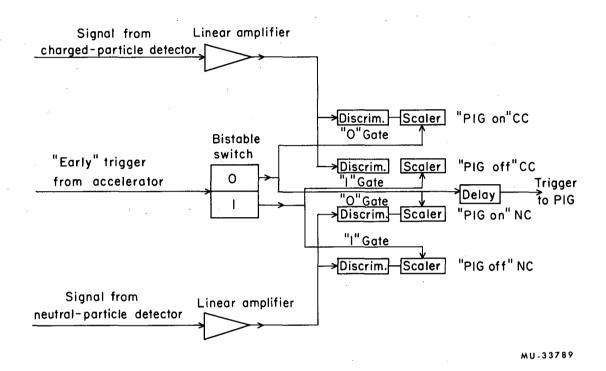
Fig. 15. Block diagram of the gating circuit used to separate out the effects of neutral collisions from the plasma target.
