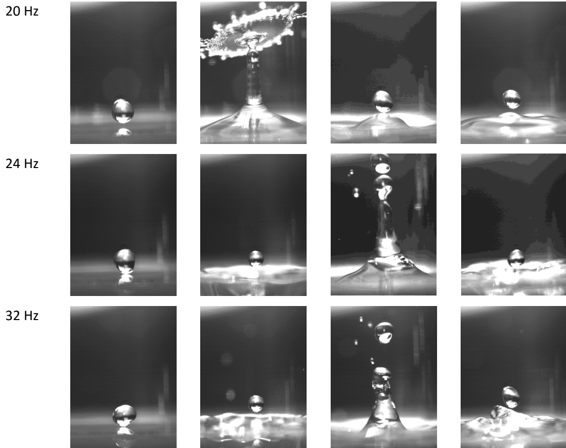
Figure 2.49. Still frames of successive droplet impacts on an H^* = 2 with We = 270 . f = 20, 24, and 32 Hz.
