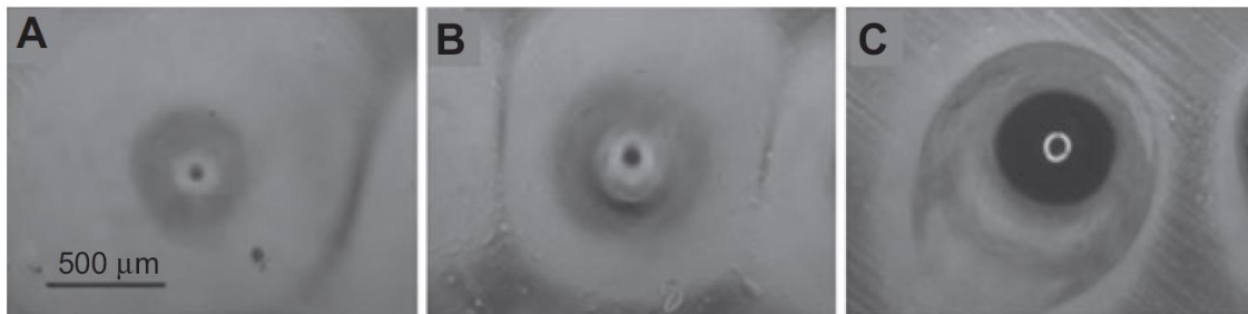
Figure 3.29. Holes on agar gel (5% concentration) for identical irradiation and varying solution thickness. (A) 300 μm, (B) 200 μm, and (C) 100 μm.
