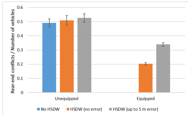
Figure 4.9: HSDW results (Heavy traffic, 100% DSRC-equipped)
