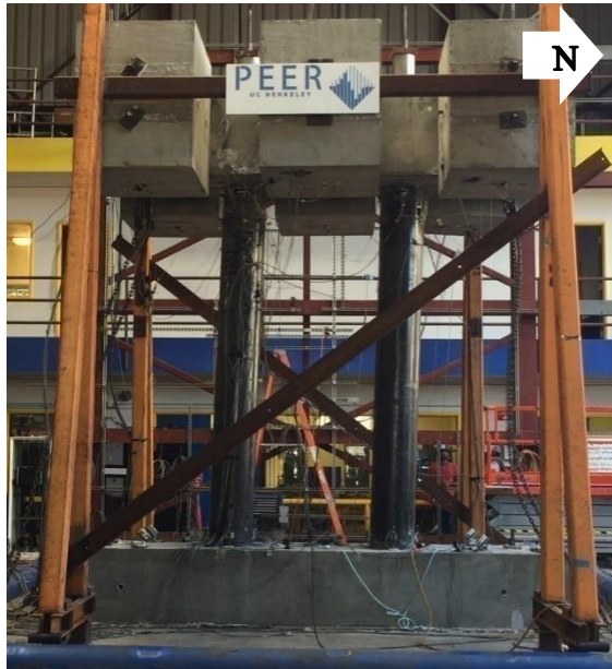
(f) Specimen deformation, \Delta=-3.5\%
