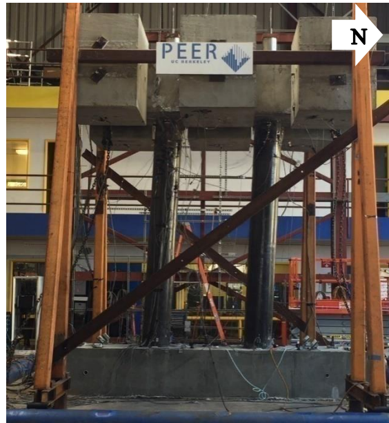
(f) Specimen deformation, \Delta=-4.5\%
