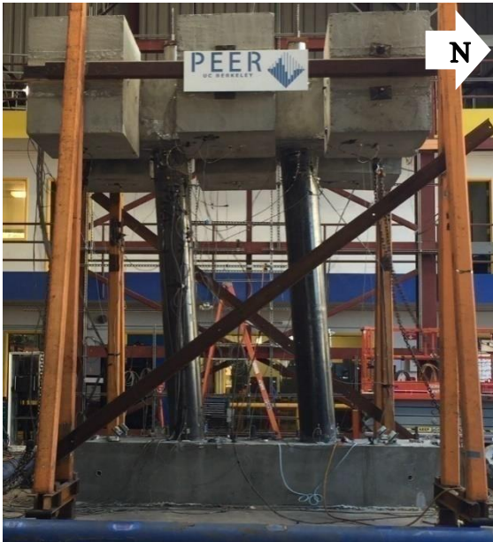
(e) Specimen deformation, \Delta=7.2\%
