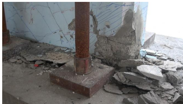
Figure 3.39 North wall damage during Phase III
