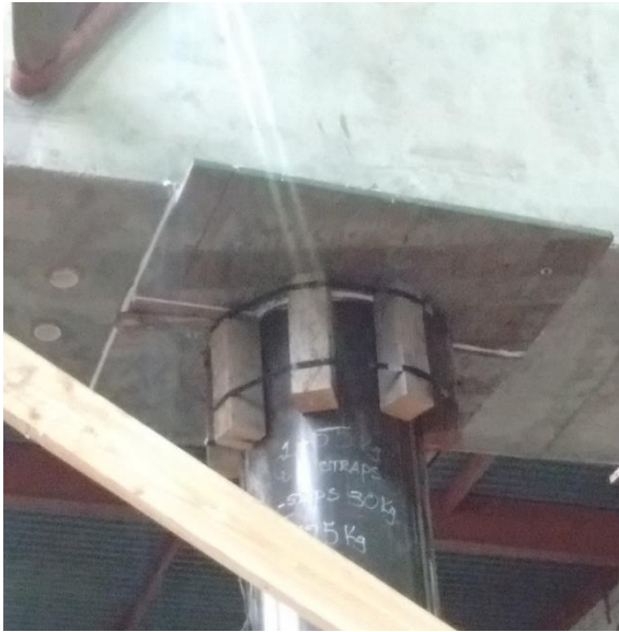
(a) Cap-beam socket seal
