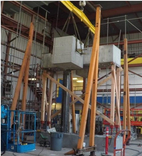
(a) Inertia block installation
