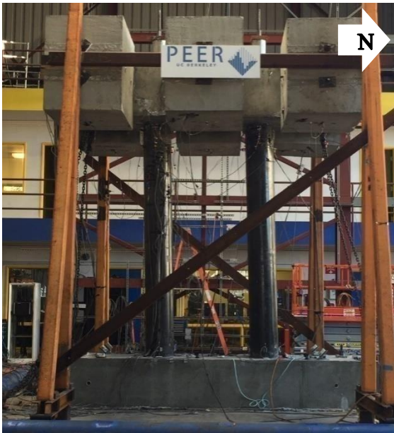
(e) Specimen deformation, \Delta=3.2\%
