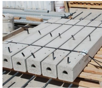
(c) Finished columns ready for transport
