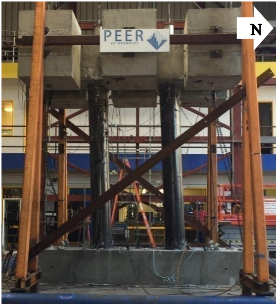
(e) Specimen deformation, \Delta=3.8\%
