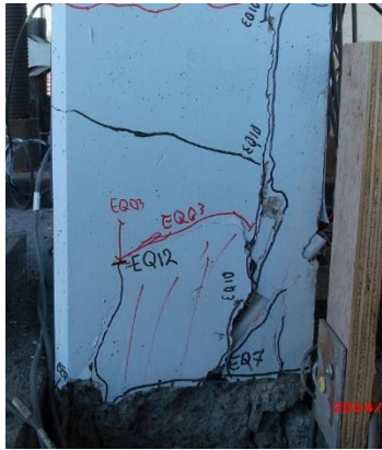
Figure 3.38 North wall damage during Phase II
