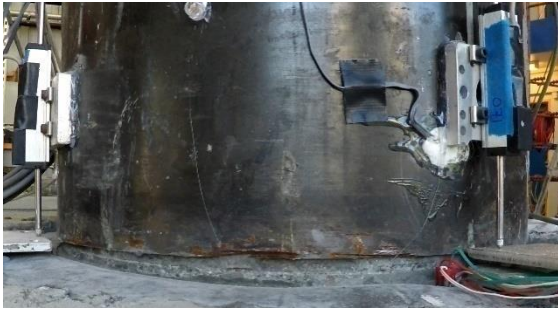
(a) South column interface, North face, \Delta=3.8\%
