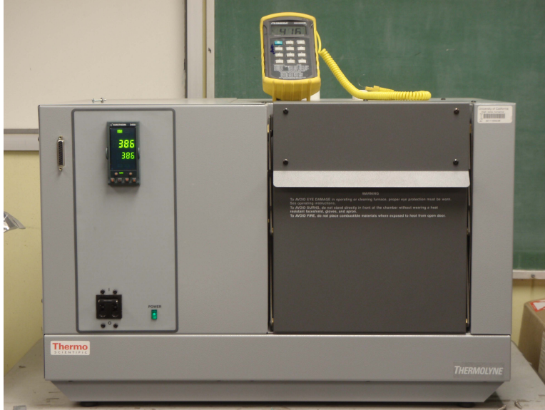
Figure 4.12: The Thermo Scientific Thermolyne furnace used for the high temperature aging of bonded samples operated in atmospheric conditions and enabled the use of an external thermocouple to monitor the temperature inside the chamber.
