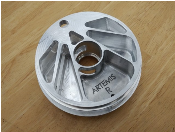
(c) Knee output carrier to linkage
