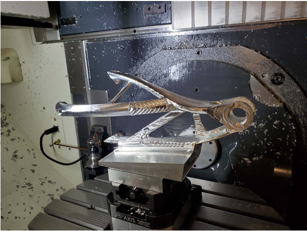
(b) Finishing section by section
