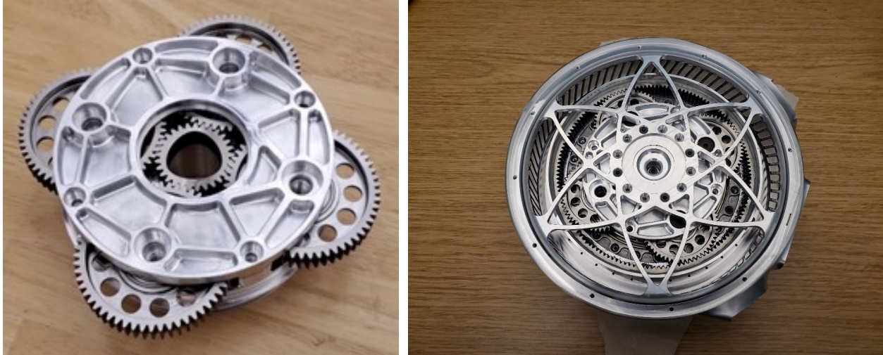
(a) custom planetary gearbox
