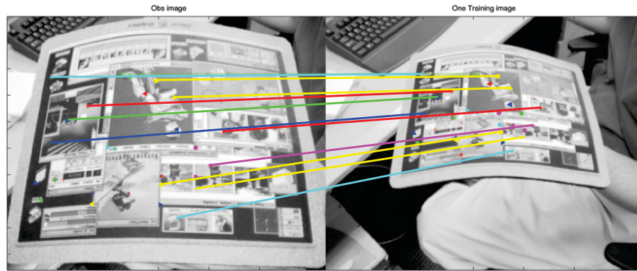
Fig. 3. Translational + KPCA: Matching using a non-planar surface undergoing warping and scale changes. During training, the object was moved away from the camera and deformed. (Left) shows the first image of the training sequence. (Right) shows the test image, which is outside of the training sequence. The shapes and colors indicate the corresponding points. In this example, 50 feature locations were correctly matched, with 10 false positives. Some lines between matches are included for clarity.
