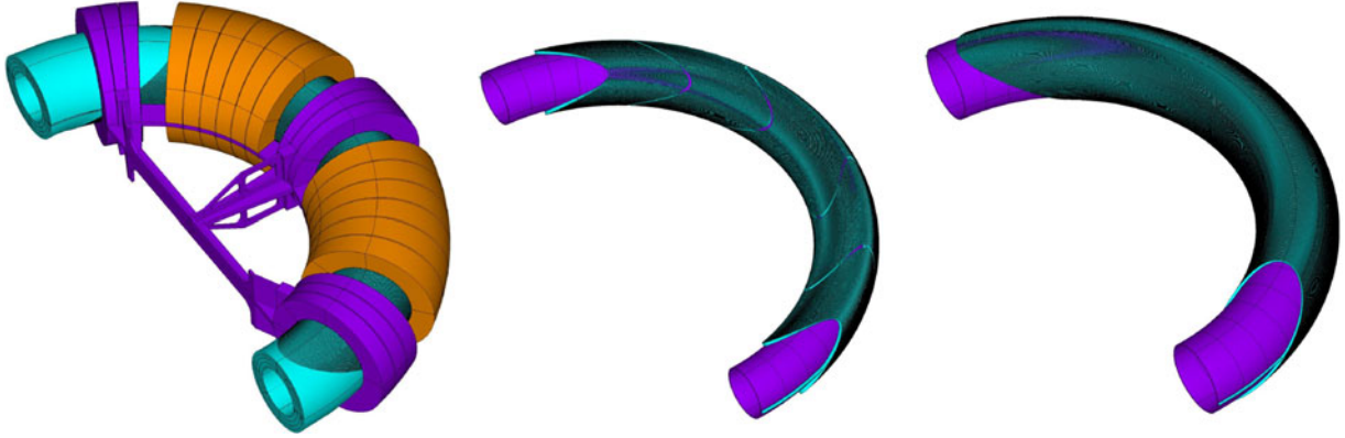
Fig. 6. Full ANSYS model with four layers and an external structure is shown on the left (the additional surrounding air needed for the magnetic model is not included). The central and right-hand figures respectively show a quadrupole and dipole conductor layer extracted from the full model (with their laminated spars underneath).
