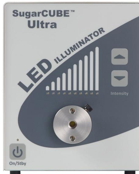
Figure 32: Adjustable light source (SugarCUBE LED fiber optic, The Ushio America Inc.)
