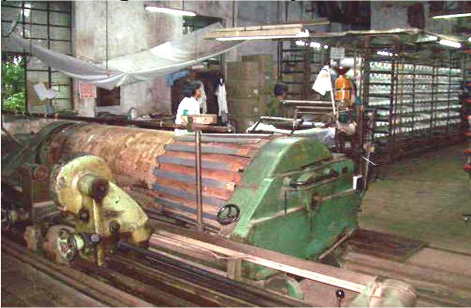
(1) Winding the yarn thread onto the warp beam
