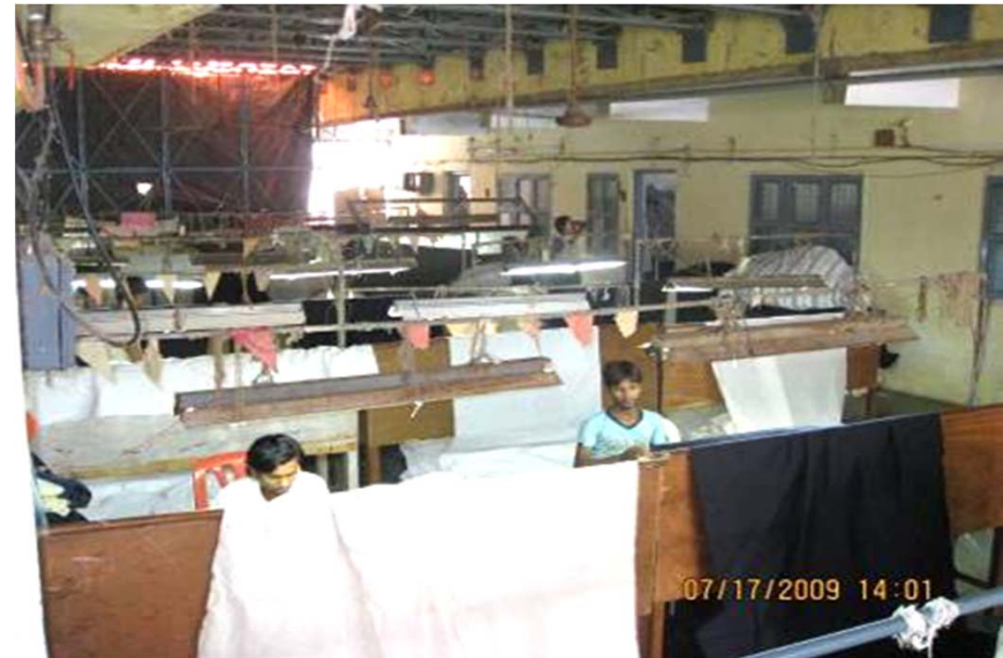
Workers spread out cloth to spot defects
