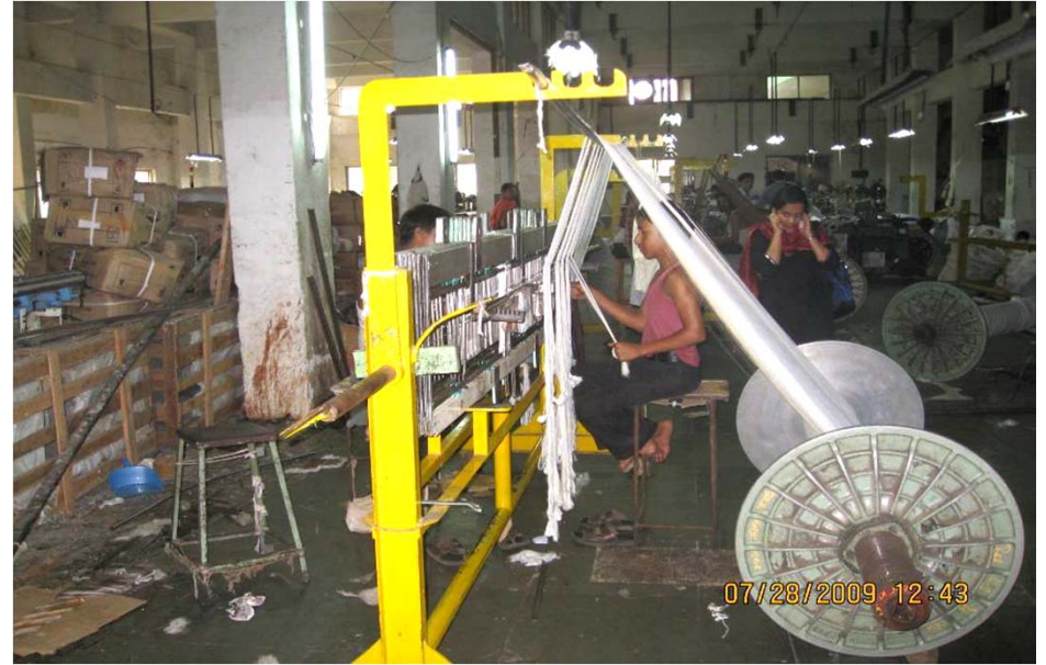
(2) Drawing the warp beam ready for weaving
