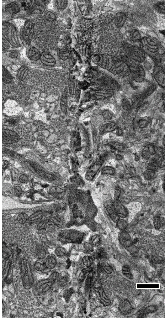
Figure 5. Cutting artifacts. Cutting artifacts are caused by softness in the plastic block. Here, a region of overlap between two tiles was softened due to dwell time being too long. Neighboring regions are unaffected as they only experienced half the beam dose. Scale bar 500nm.
