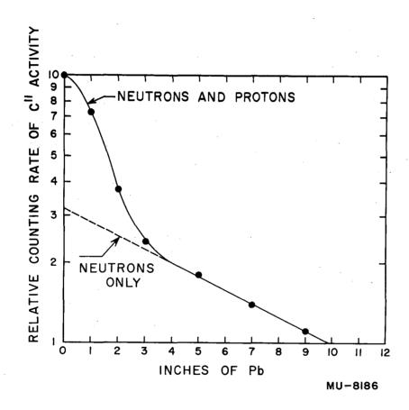
Fig. 4 Determination of the neutron-proton ratio at the detector foil position. Linear extrapolation of the neutron attenuation curve in Pb shows that the neutrons comprised 32 percent of the total activity observed.
