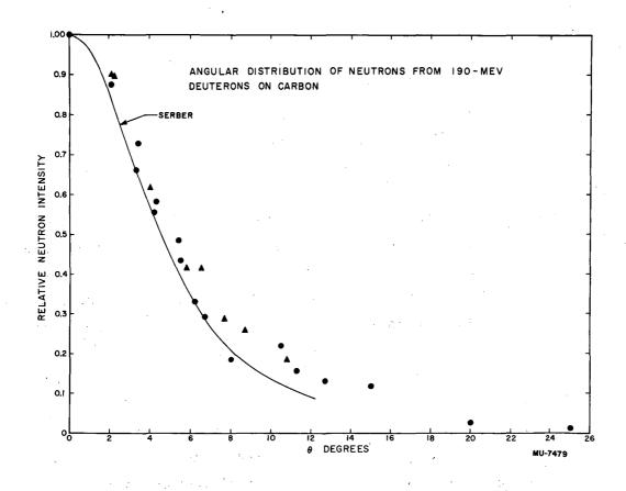
Fig. 3 Angular distribution of neutrons from deuteron stripping in carbon. The triangles and circles represent vertical and horizontal distributions, respectively.
