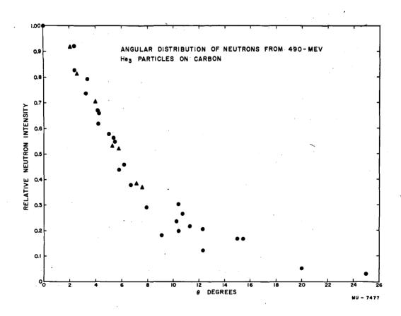
Fig. 5 Angular distribution of neutrons from He<sup>3</sup> stripping in carbon. The triangles and circles represent vertical and horizontal distributions, respectively.
