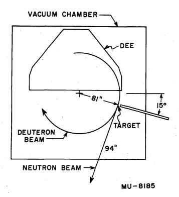
Fig. 1 Experimental arrangement. The carbon detector foils were placed on the outer surface of the vacuum chamber wall.
