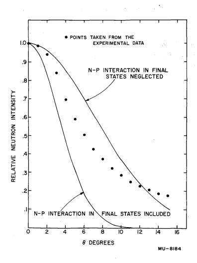
Fig. 6 Theoretical angular distribution of neutrons from He<sup>3</sup> stripping.
