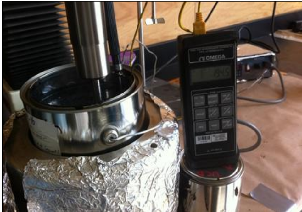
Figure 7.1 Mixing apparatus for asphalt rubber binder.
