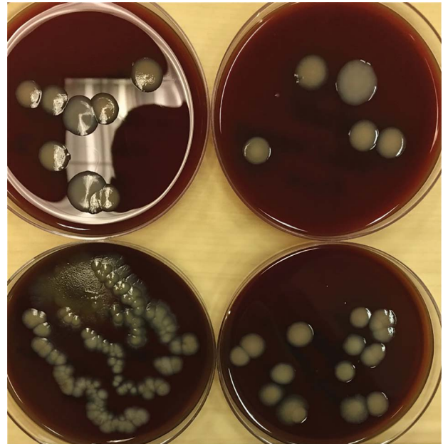
Figure 5. Culture of a new STATIM autoclave reservoir from a different surgery center after 20 days on initial use. The reservoir wall from a STATIM autoclave purchased as part of another study and not yet exposed to the boiling water protocol, was cultured after 20 days of use. These plates were incubated for 7 days and demonstrated contamination. 35
