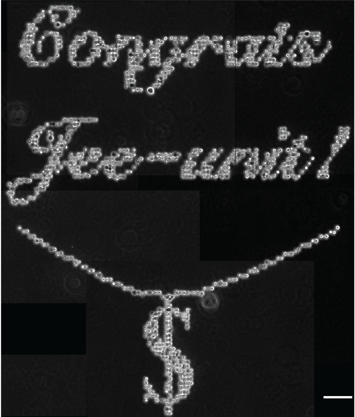
Figure 3-2. Micron scale artwork. Any conceivable artwork can be rasterized and patterned via cell “pixels” to create micron-scale cell-based art. Scale bar is 100 \mu\text{m} .
