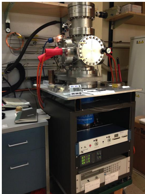
Figure 29: The custom-built thermal evaporation system constructed in collaboration with Cho and Cybart, note the high current cables for two centralized evaporation sources coming through the left and right side of the chamber. The sample is mounted onto the flange capping the top of the chamber.
