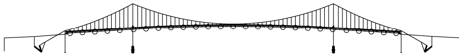
Fig. 4. Locations of spatially discretized aerodynamic forces (“aerodynamic” nodes) along the bridge deck
