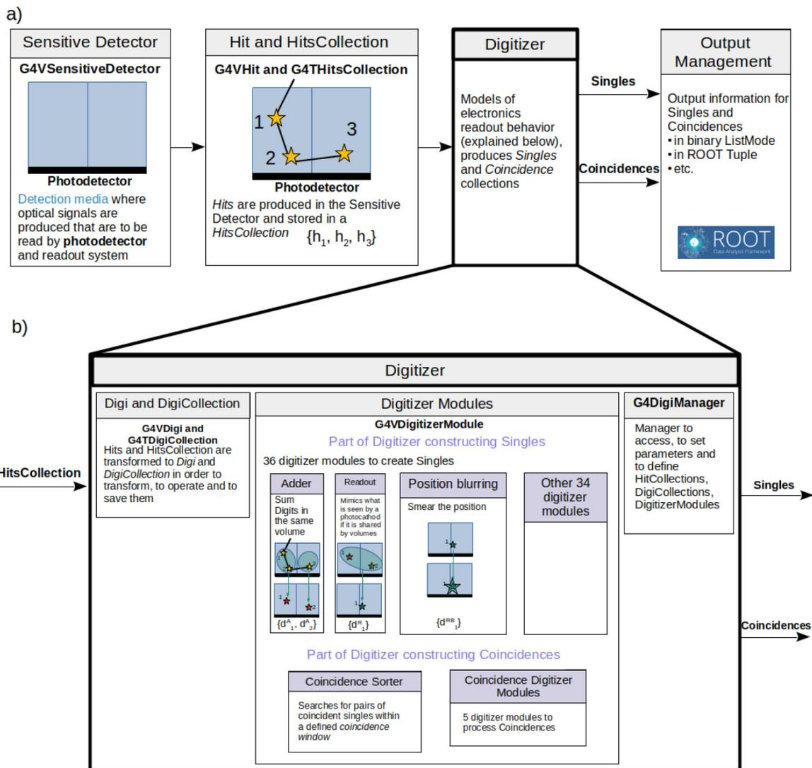
**Figure 3.** A schematic of the GATE digitizer main workflow and elements: a) digitizer module within the GATE environment and its interaction with other modules; b) digitizer module. An example of a scintillation detector containing two scintillation crystals and a photocathode is illustrated.
