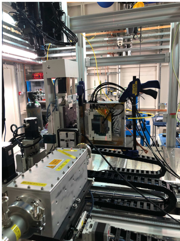
Figure 8. The module in place at the beamline during coarse alignment. The opaque front of the test box has been removed. The data, power and magnetic field probe cables can be seen entering the box from the top with a nitrogen pipe (yellow) entering on the right. The magnetic field probe is taped in place over the module and the red horizontal laser alignment beam can be seen.
