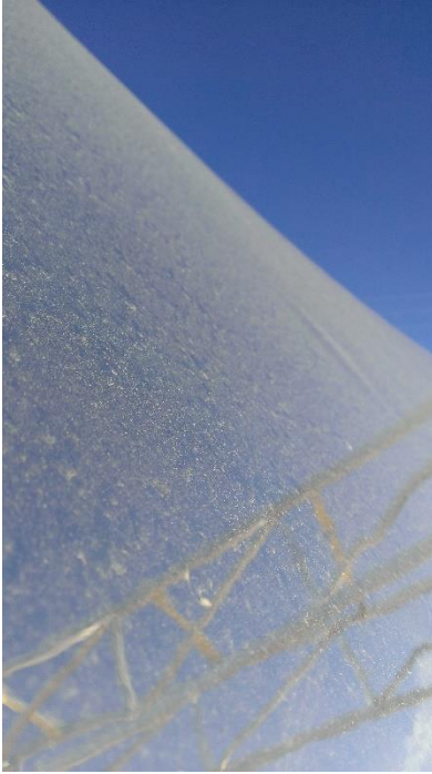
Primary Mirror Surface is slightly dusted, causing scattering of light on its way to the receiver
