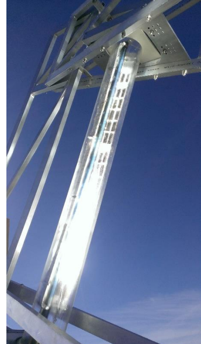
Condensation causes significant reflection / scattering when illuminated
