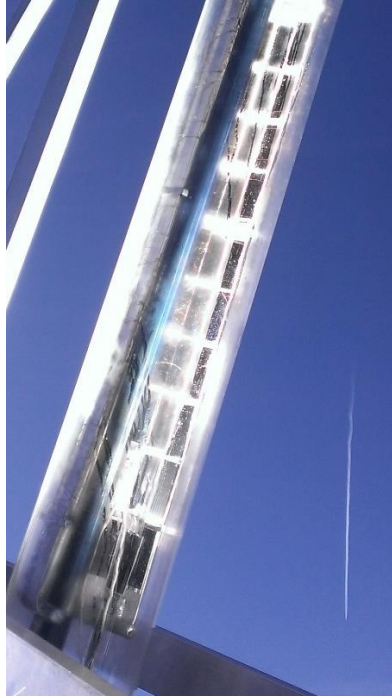
Condensation formed on inside of tube
