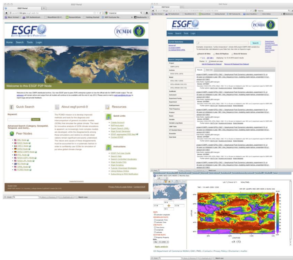
Figure 15. The ESGF node installation script deploys the home page of a minimally configured Web front-end application, shown at left. Included on the home page are search capabilities, information pertaining to the node and organization, quick links to commonly used tools, links to other ESGF nodes, and analysis tools. Example search page and analysis/visualization results are shown on the right.
