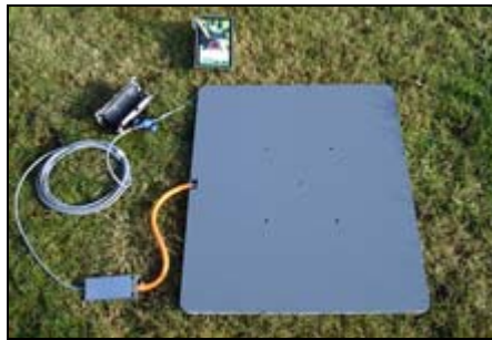
Figure 5.1: Piezoelectric pad counter (Eco-Counter)
