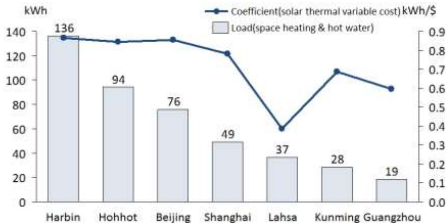
Figure 27 – Impact of heating load on solar thermal adoption’s sensitivity to variable cost
