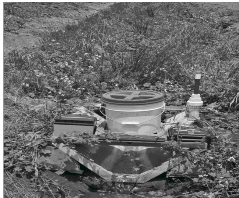
Figure 16. Anderson trial showing vegetated ditch and electronic dosing unit, 2008. Photo by B. Anderson
