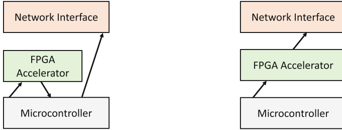
(a) FPGA accelerator as a separate module has higher latency and higher bandwidth requirements.
