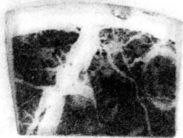
Fig. 3. Sample slide of CA-Ora-244 jasper debitage (Sample 2) prepared for SEM analysis. Low magnification using SEM shows characteristic chalcedonic veins in jasper matrix.
