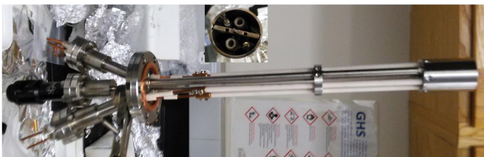
Fig B.3(A)STM4 doser loadlock system,(B)a load lock doser with water cooling, (C) a load lock doser with two crucilbe (inset) mounted.
