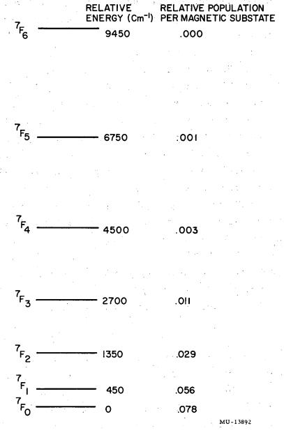
Fig. 23. Approximate <sup>7</sup>F level structure in Pu<sup>239</sup> inferred from optical spectroscopic data. The relative population per magnetic substate is calculated for 1700°C, the approximate plutonium beam temperature.
