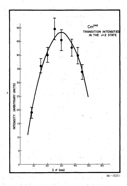
Fig. 11. Variation of resonance intensity in the J=2 state of  $Cm^{242}$  with rf current.
