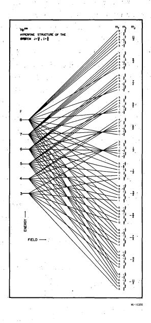
Fig. 29. Energy-level diagram of the system J = 11/2, I = 5/2 in a magnetic field (not to scale).
