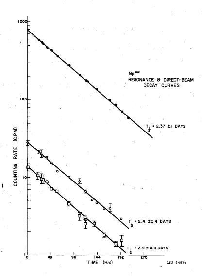
Fig. 27. Results of half-life determination of the sample.
