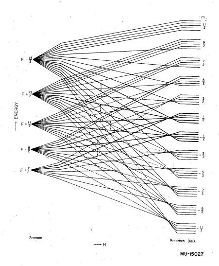
Fig. 30. Energy-level diagram of the system J = 11/2, I = 2 in a magnetic field (not to scale).
