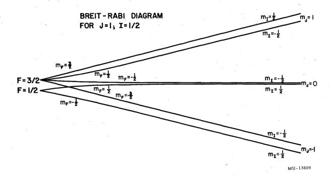
Fig. 16. Energy levels of the system J = 1, I = 1/2 in a magnetic field.
