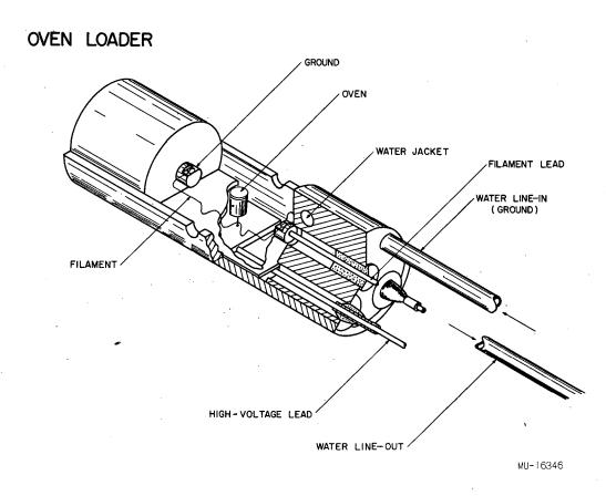
Fig. 8. Modified high-temperature oven loader used in researches at  $2000^{\circ}C$ .
