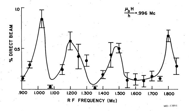
Fig. 18. Results of a very-low-field search to obtain information regarding the electronic ground state of plutonium.
