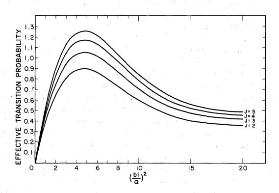
Fig. 13. Calculated transition probabilities for the four states of curium. The abscissa is a quantity which is proportional to the square of the applied rf current. The ordinate is the sum over all flop-in transitions in the particular J state, of the Majorana transition probabilities averaged over the atomic-beam velocity distribution.
