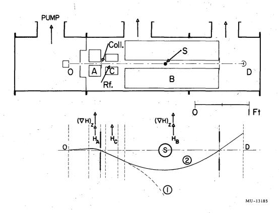
Fig. 3. Schematic arrangement and trajectory in an atomicbeam flop-in apparatus.
