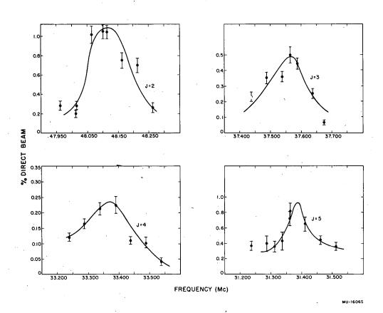
Fig. 10. Observed curium resonances at 13.4 gauss.
