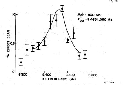
Fig. 21. (a) Data obtained during the search for  $\Delta F = \pm 1$  transitions at low field. The resonance near 8.5 Mc is due to the transition F = 3/2,  $m_f = 1/2 \longleftrightarrow F = 1/2$ ,  $m_f = -1/2$ . (b) Detail of the transition F = 3/2,  $m_f = 1/2 \longleftrightarrow F = 1/2$ ,  $m_f = -1/2$  on which the hyperfine-structure assignment is based.
