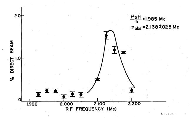
Fig. 19. Observed plutonium resonance at 1.4 gauss.
