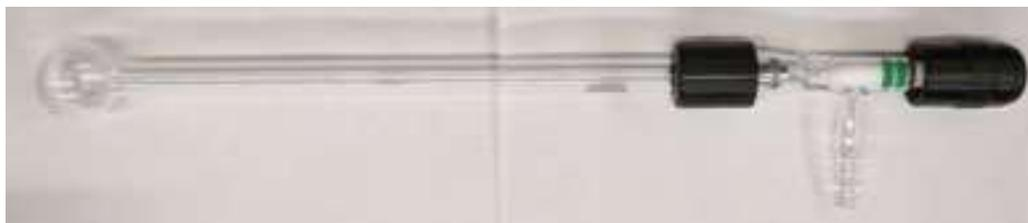
**Figure A.2:** Attachment of a Breen adapter onto a ½” ASAP tube.
