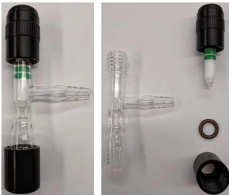
**Figure A.1:** A  $\frac{1}{2}$ " Breen adapter (left), and the adapter disassembled into its four components (right).
