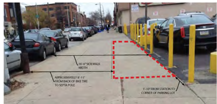
Philadelphia Bike share, Site plan configuration for the Standard bike share stations; the equipment is the same as what will be implemented in Downtown Los Angeles.
