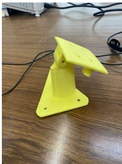
Figure 5.2: Adjustable AOA fixture
