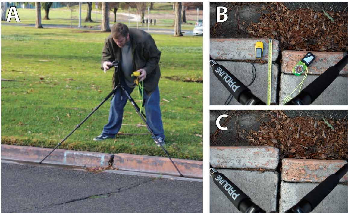
Figure 3.2: (A) The original setup to photograph an offset curb in 2009–2010 (after Funning et al., 2010) in which the camera is centered, leveled, and positioned 1 meter above the curb. Two photographs were taken; (B) one with a tape measure for scale, a portable GPS, and a compass and (C) one with nothing.
