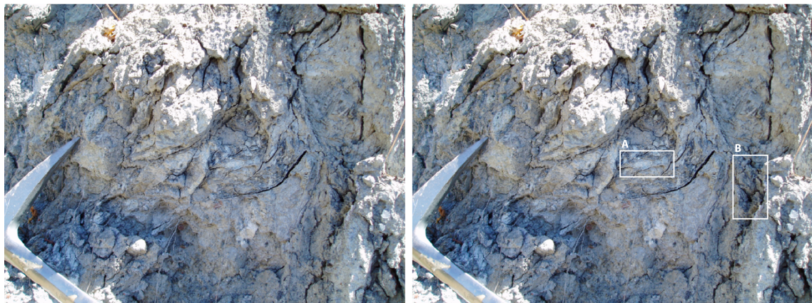
Figure 4.3: Close-up of the fault gouge showing the heterogeneous fine-grained matrix; darker colored gouge is the talc-chlorite-tremolite assemblage (example: inset B), lighter colored gouge is the antigorite serpentinite (example: inset B).
