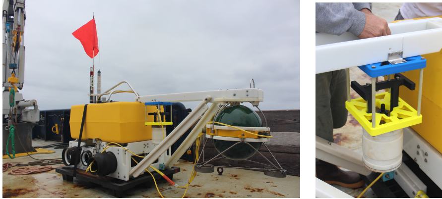
Figure A.8: Photos of the DPG drop mechanism. The left photo shows the location of the DPG drop on the OBS package, and the right photo shows a close up of the DPG during deployment, before the release..
