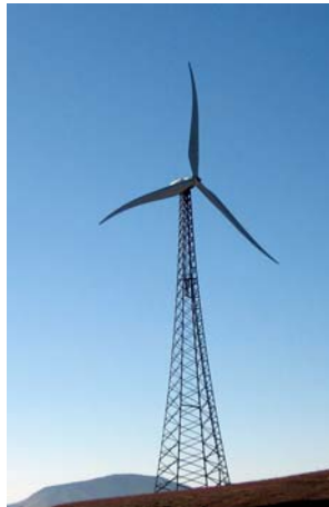
Figure 6.9. DOE Knight & Carver STAR (Sweep Twist Adapted Rotor) blade design in field testing in Tehachapi. Co-developed by UC Davis/CWEC.
