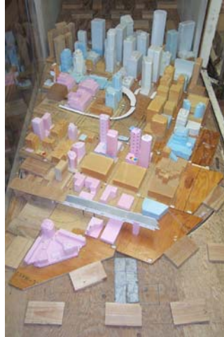
Figure 6.7. Wind-tunnel test setup for urban wind resource assessment.
