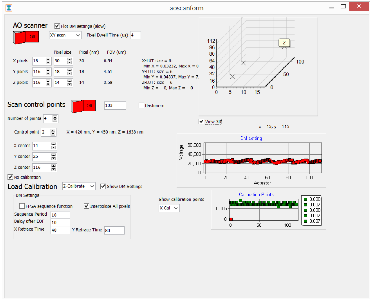
Figure 2.11: SimFCS module for deformable mirror based scanning. The module allows frame scanning (“AO scanner”) in x-y, x-z, y-z, and x-y-z. The “Scan control points” button allows the selection of any number of locations in the region (shown in graph on the top right), then the DM will cycle through the list of points, parking the beam on each location for some amount of time.
