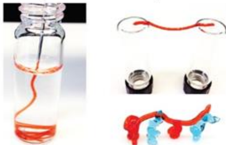
Figure 23. Gel prepared by combining silicate nanoplatelets and gelatin. Reprinted with permission from ACS Nano, Vol. 8, Issue 10, AK Gaharwar, RK Avery, A Assmann, A Paul, GH McKinley, A Khademhosseini, BD Olsen, Shear-Thinning Nanocomposite Hydrogels for the Treatment of Hemorrhage., 9833–9842. Copyright 2014 American Chemical Society.(124)
