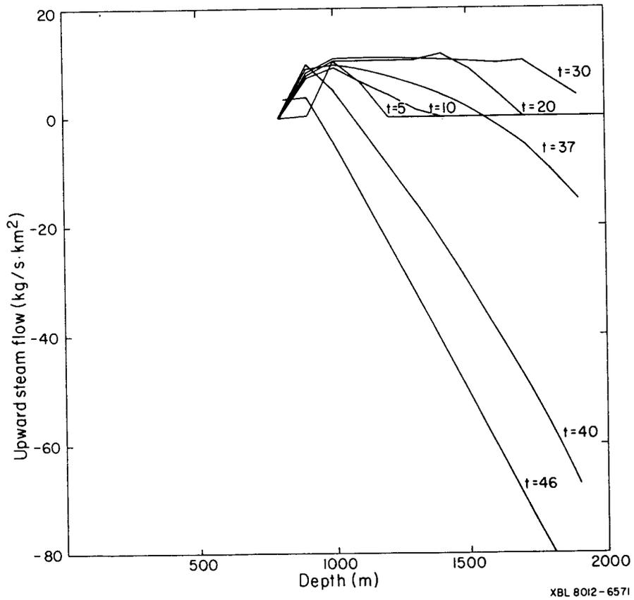
Figure 2. Steam flow in the reservoir at various times.
