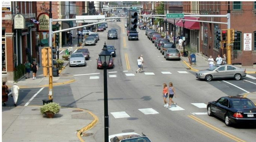
FIGURE 24: EXAMPLE CURB EXTENSION
