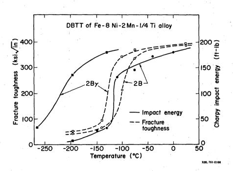
Fig. 1. Temperature variation of fracture toughness and Charpy impact energy in 8Ni steel.
