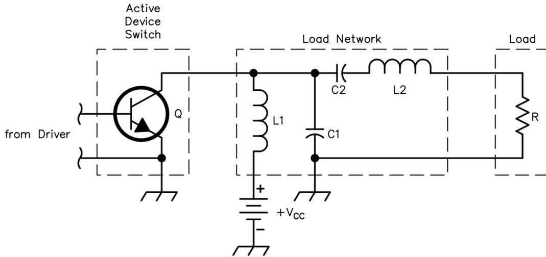
Figure 3.8: Class E Amplifier Schematic
