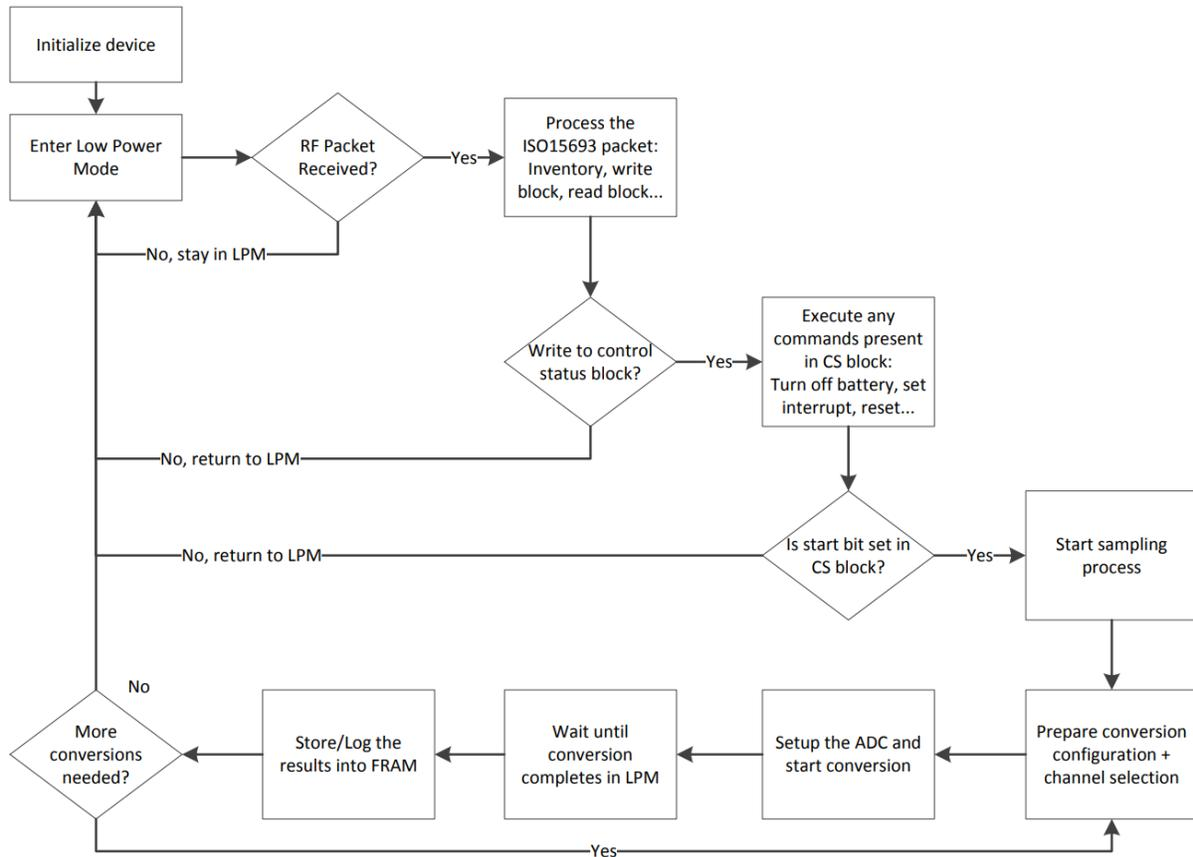
Figure 3.6: RF430 Firmware Flow
