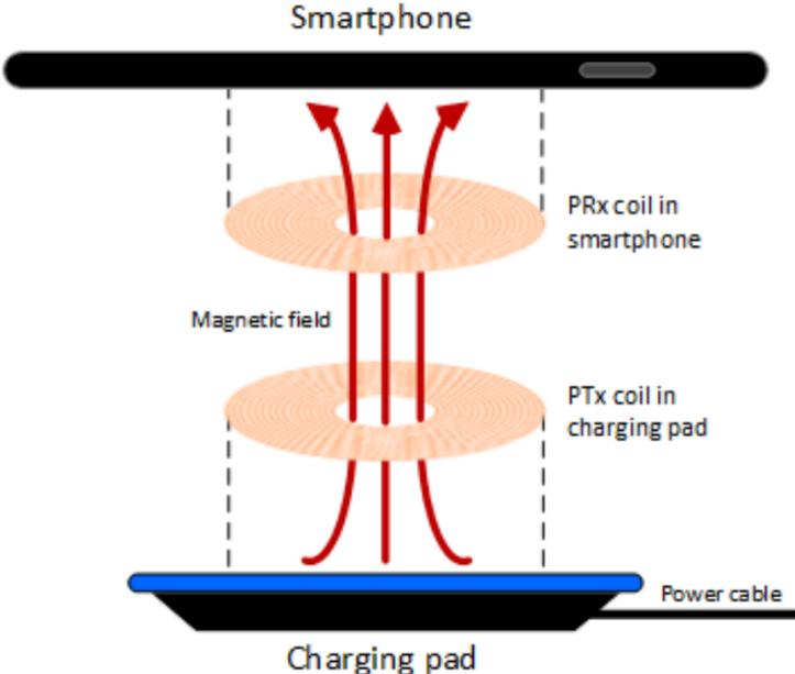
Figure 1.2: Qi Wireless Power Transfer [7]
