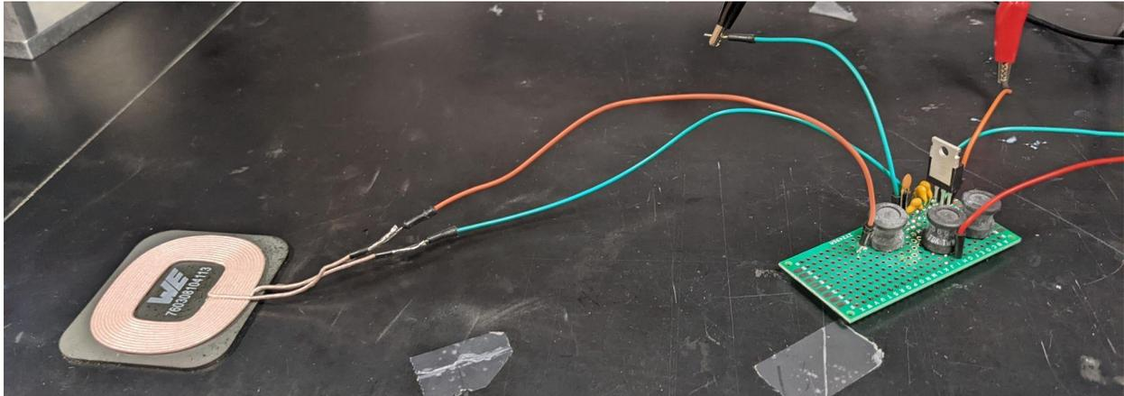
Figure 3.10: Class E Amplifier on Protoboard
