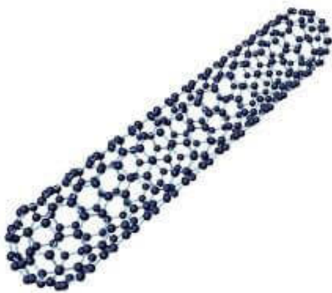
Figure 4.1.1 Single Walled Carbon Nanotube 4
