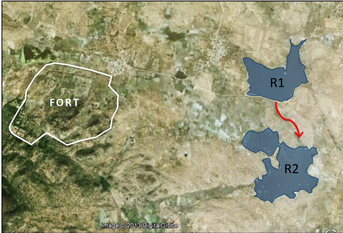
Fig. 6-19: Reservoirs R1 and R2 with respect to the fort at Maliabad. R1 and R2 are connected such that excess water from R1 gets transported to R2.
