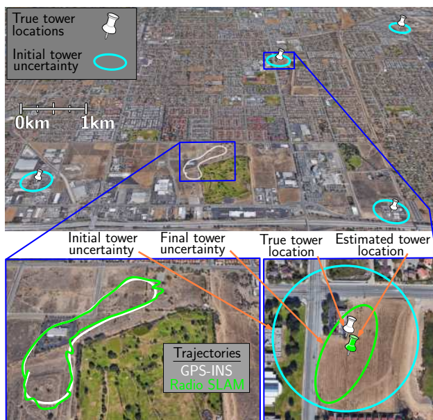
Figure 3.5: Environment layout and experimental results showing the estimated UAV trajectories from (i) its onboard GPS-INS integrated navigation system (white) and (ii) radio SLAM (green), the initial position uncertainty of each unknown tower, and tower 1 final position estimate and corresponding uncertainty ellipse. Image: Google Earth.
