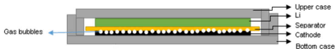
Figure 2.5 Schematic of GGA working mechanism
