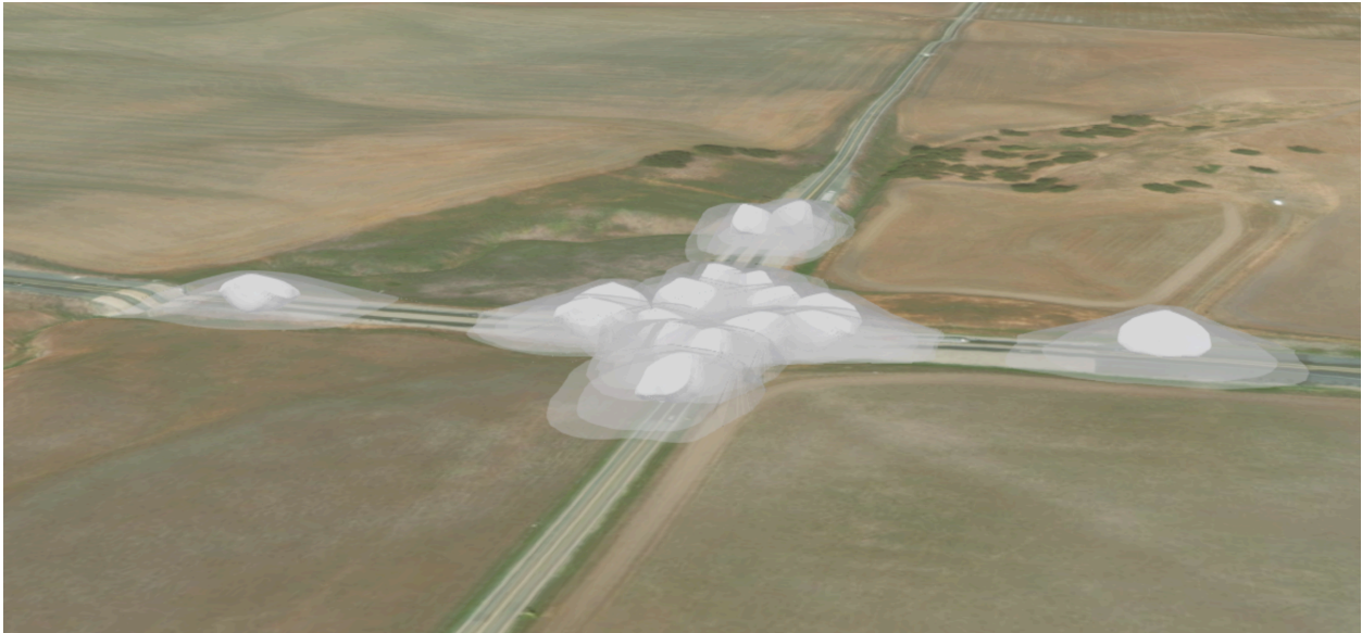
Figure 40. Example of GIS-native calculation of light volumes at 0.1, 1, and 10 lux (horizontal) for the 12/113 roundabout, produced by EvariLux.
