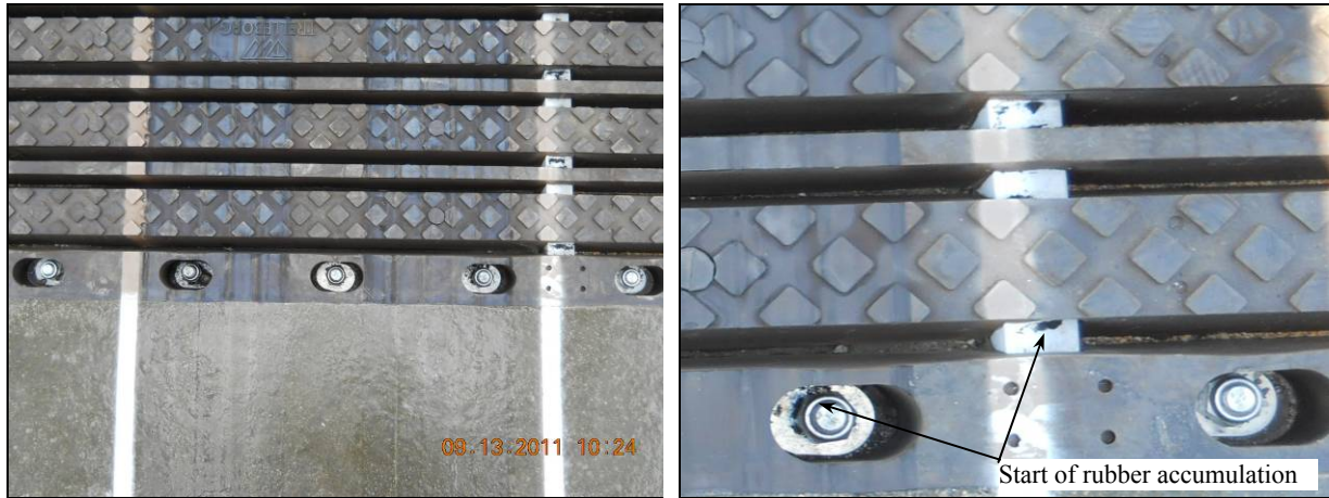
Figure 4.10: Phase 1.1: Rubber abrasion on Trelleborg unit after 100,000 load repetitions.
