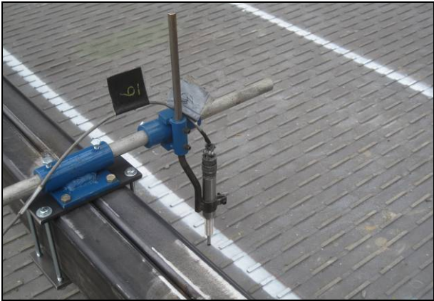
Figure 3.7: LVDTs on edge of steel plate. (Instrument #5)
