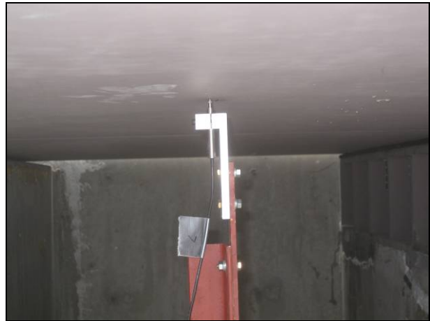
Figure 3.11: LVDT on bottom of steel plate. (Instrument #13)
