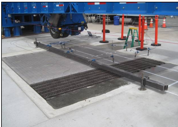
Figure 2.12: HVS on test structure prior to start of testing.
