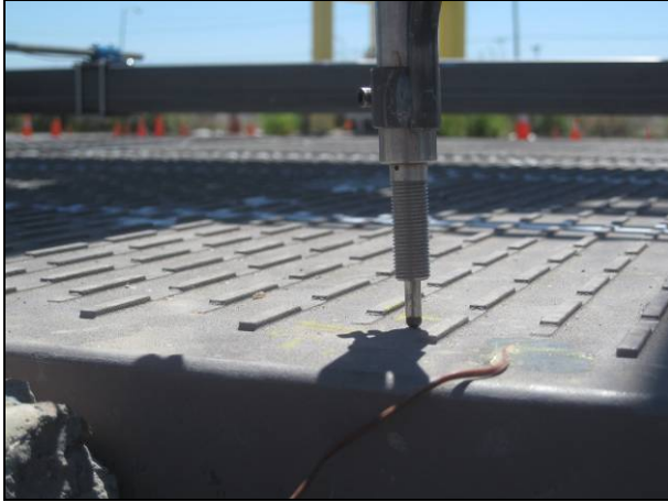
Figure 3.8: LVDTs on edge of steel plate. (Instrument #6)
