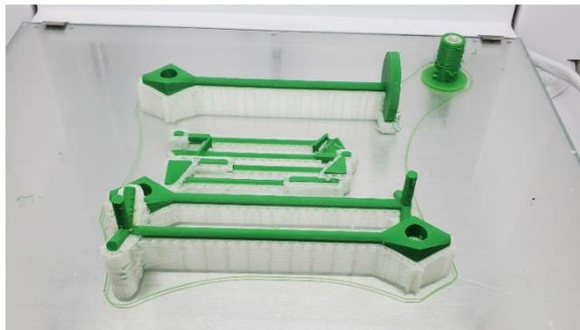
upright without total failure or *Figure 3.2: Successful model print layout*
