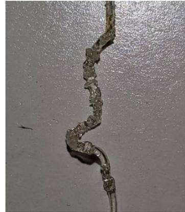
*Figure 3.3: Ultimaker PVA, damaged by humidity*
