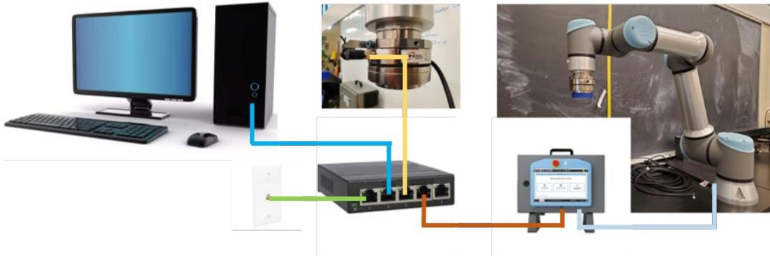
Figure 4.4: Ethernet connection system for UR16e and Axia F/T sensor.
