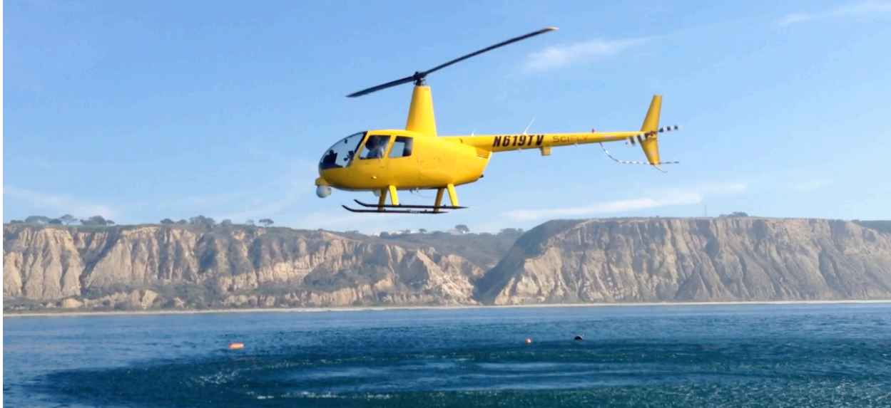
Figure 5.1: The Robinson R44 helicopter hovering above the sensor station at end-fire to the array during the head-wave experiment.
